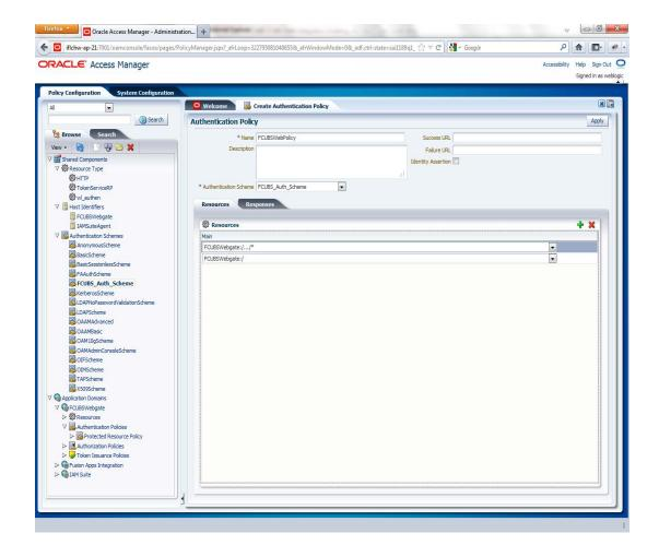
Add DN in the Responses section. Enter the value as **\$user.attr.dn**. The responses maintained in the tab will be added in the response header during the authentication.
