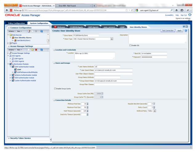
3. After input of the above information click on 'Apply' button. On successful creation, click test connection button to verify whether the LDAP connection is working fine.
