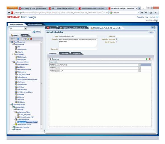
Add DN in the Responses section. Enter the value as **\$user.attr.dn**. The responses maintained in the tab will be added in the response header during the authorization.
